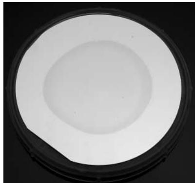
Figure 2-6: Contamination during warming-up observed on a 4" Pt wafer heated up to 700°C for 1 min.
